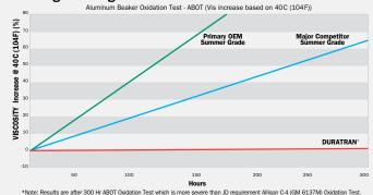
If the heat doesn't get you, oxidation will. To benefit from truly long-life performance your Transmission/Hydraulic Fluid has to resist oxidation degradation. DURATRAN's advanced formulation keeps its "fresh oil" properties longer than leading competitors. And that gives you increased productivity you can profit from.
